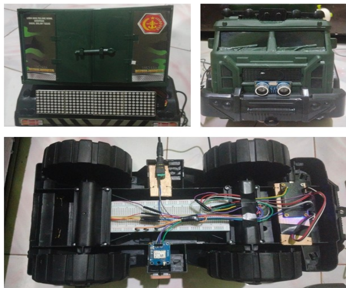
Figure 5. Vehicle detection device circuit in displaying information
